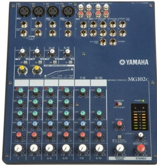
**The Mixer Board channel controls** (the only thing you should touch on the sound board)
